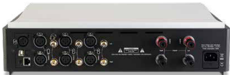
ABOVE: Three analogue ins on RCAs and XLRs (switched) are routed via optional phono or line stages. Digital module [far left] includes Toslink optical and AES/EBU (to 192kHz/24-bit) plus USB-B and Ethernet (384kHz/32-bit and DSD512). The speaker outputs are on Furutech 4mm terminals wired internally with Kubala-Sosna cable
